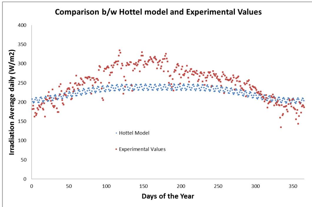
Fig.2 Comparison between Hottel's model and Experimental values
