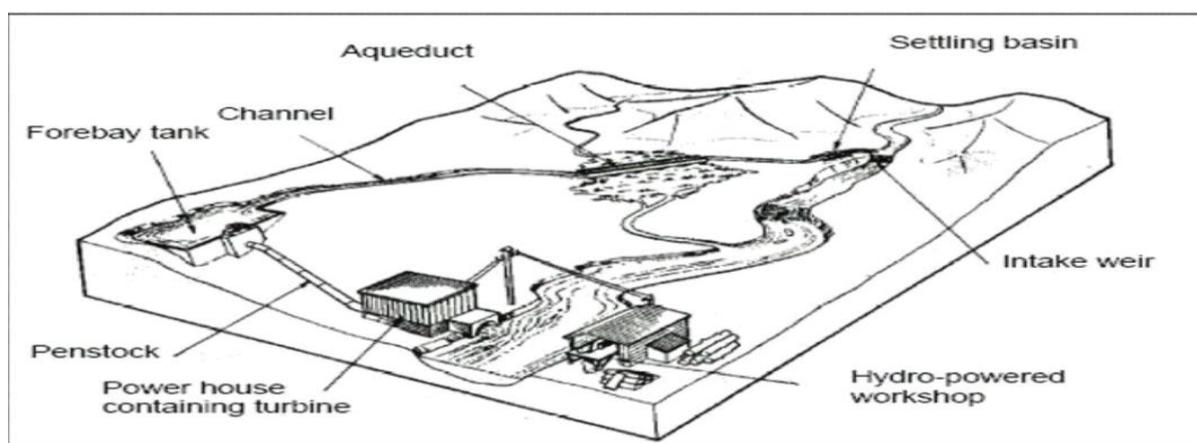
**Figure 1:** Layout and components of a typical micro hydropower installation [9].
