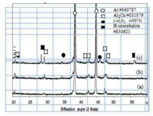
Figure 2. X-Ray diffraction patterns of Al-4wt.%Cu / 15vol.% Silica (a) as-sintered, (b) as-forged, (c) as-heat treated.
