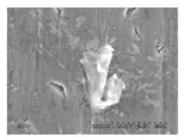
Figure 4. SEM image of remaining silica shown as bright irregular particle surrounded by reacted area (Al-4wt%Cu /15vol%Silica: Sintering 650°C -1h
