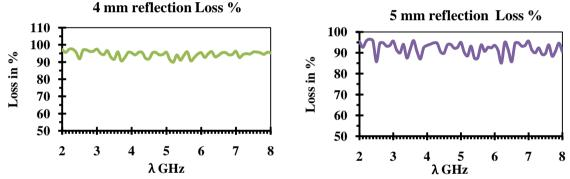
Fig. 7: Reflection Loss in % of 4mm thicknessFig. 8: Reflection Loss in % of 5mm thickness
