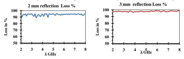
Fig. 5: Reflection Loss in % of 2mm thickness Fig. 6: Reflection Loss in % of 3mm thickness
