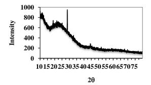
Fig. 4:XRD spectrograph of CNM with decorated nickel
