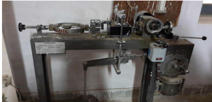
Figure 2 – Direct Shear Test Apparatus
