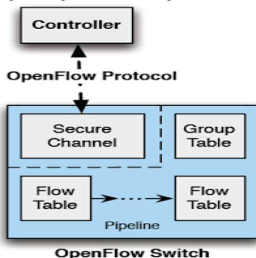
**Fig. 5 Open Flow Switch**
