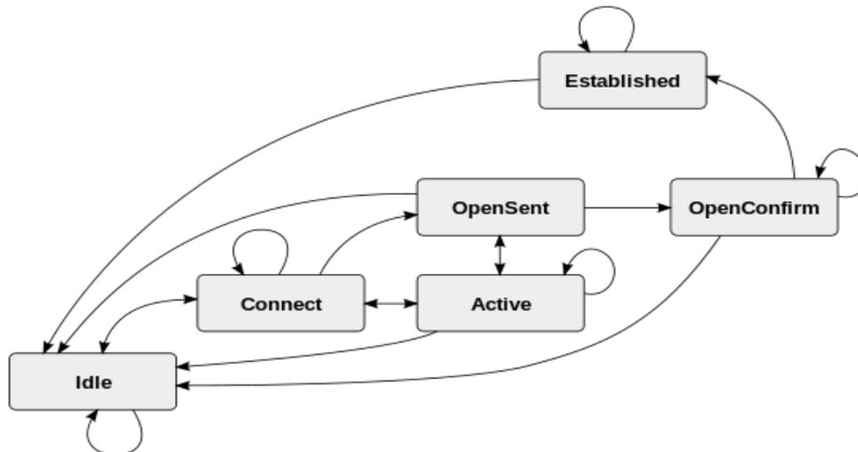
**Fig. 3 BGP Finite State Machine[8]**
