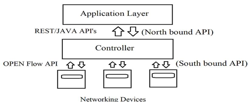
**Fig 4. Open SDN Architecture**
