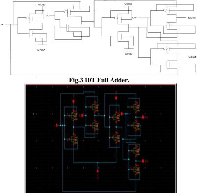
Fig.4. Schematic of 10T Full Adder.
