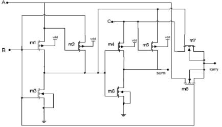
Fig 5. 8T Full adder with FinFETs.
