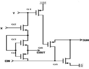
Fig 7. 6T Full Adder with FinFETs.
