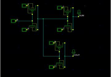
Fig 8. 6T Full Adder with FinFETs
