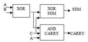
Fig.2 Basic Design Approach for Hybrid Full Adder.
