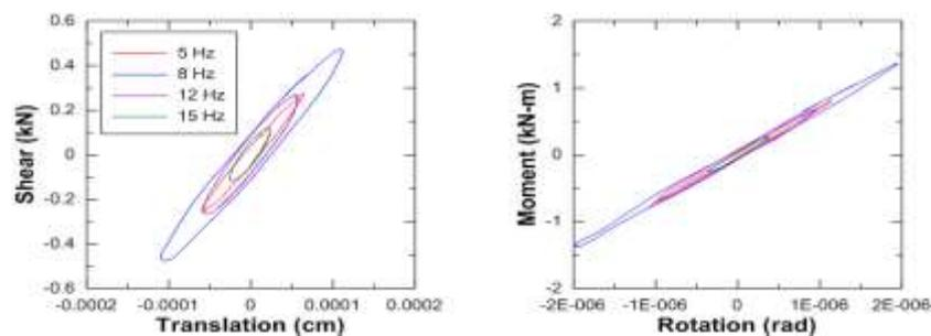
**Figure 7:** Shear versus base-sliding-displacement and moment versus base-rotation response of unbraced structure with shaking in transverse direction at GVDA site.
