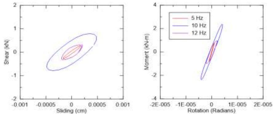
**Figure 5.** Shear versus base-sliding-displacement and moment versus base-rotation response of braced structure with shaking in longitudinal direction at WLA site
