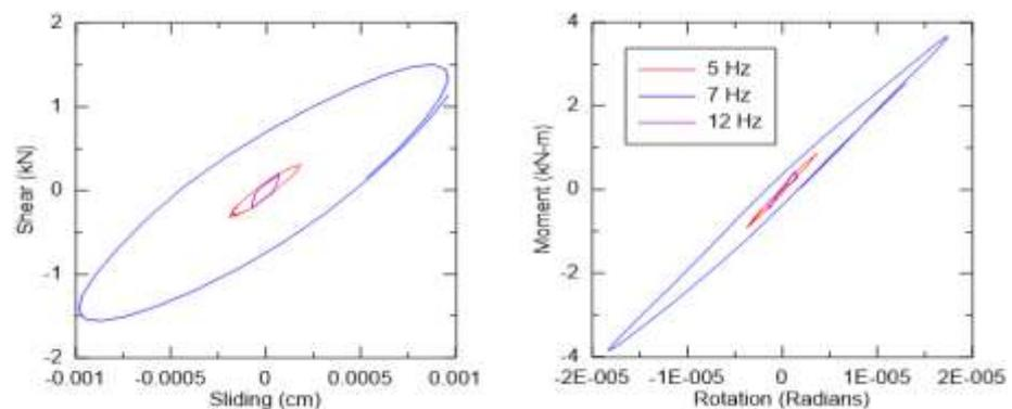
**Figure 4.** Shear versus base-sliding-displacement and moment versus base-rotation response of unbraced structure with shaking in transverse direction at WLA site
