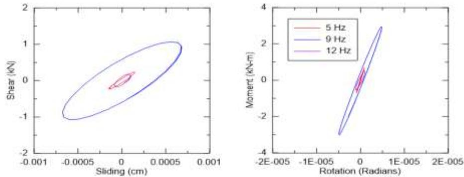
**Figure 3.** Shear versus base-sliding-displacement and moment versus base-rotation response of unbraced structure with shaking in longitudinal direction at WLA site.
