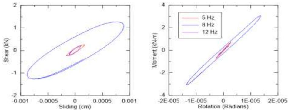
**Figure 6.** Shear versus base-sliding-displacement and moment versus base-rotation response of braced structure with shaking in translational direction at WLA site
