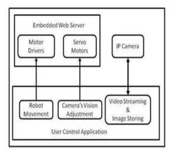
Fig. 9 Association of Embedded Web Server and User Control Application
