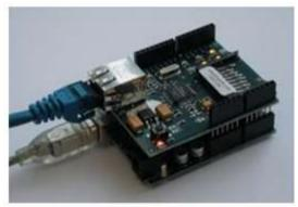
Fig.5 Arduino Duemilanove and Ethernet Shield
