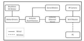
Fig.2 Functional Block Diagram of the Design
