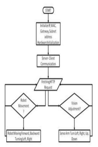
Fig. 8 Flow Chart of Embedded Web Server
