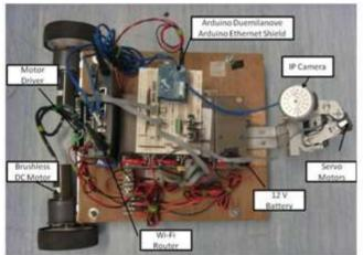
Fig. 3 Wi-Fi Surveillance Robot
