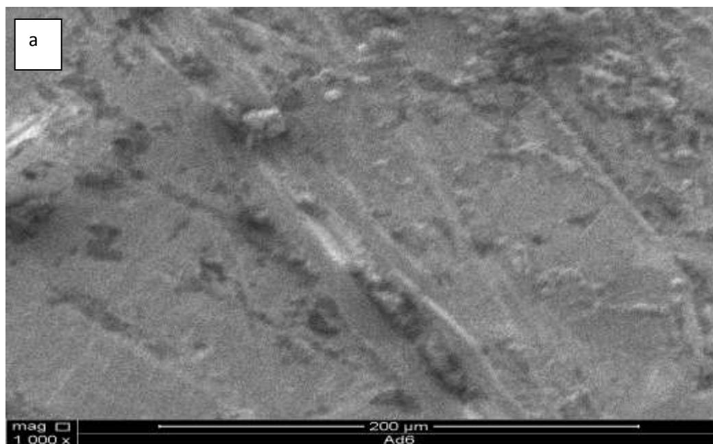
Fig. 8 SEM images of the mild steel surface before (a) and after (b) immersion in 1 M HCl solution containing 1000 mg/L of PM extract.
