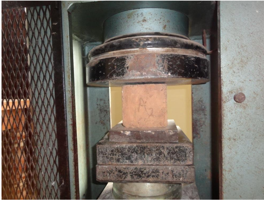
Plate 1: Compressive test of 100mm cube
