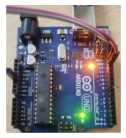
It goes about as an interface. Outer (non-USB) power can come either from AC to DC connector (divider mode) or battery. The connector can be related by halting 2.1mm center positive fitting into the boards ability jack. Leads from the battery can be implanted in the Gnd and vin stick header of the power connector.
