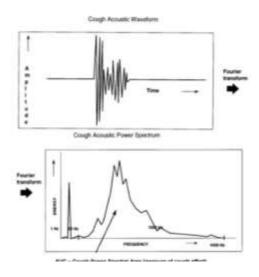
This cough acoustic waveform is used to computerized system that quantifies the energy expanded in a cough by digitizing the audio signal and measuring the time under the transform. The graph shows that the computerized cough acquisition and analyze system are a valid and methodology for evaluating cough associated patients.
