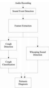
An algorithm for automated diagnosis of pertussis using audio signals by analyzing cough and whoop sound is presented.
