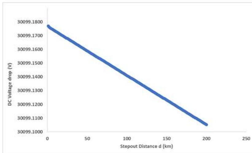
**Figure 3.5:** dc voltage drop for 1km to 200km under load condition for akpo field.
