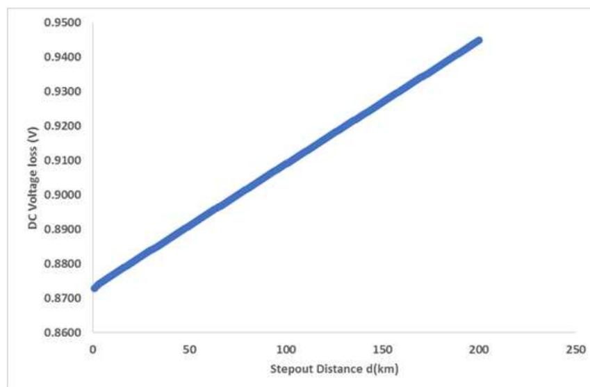
**Figure 3.6:** dc voltage loss for 1km to 200km under load condition for akpo field.
