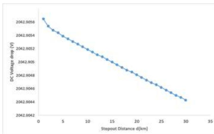
**Figure 3.3:** total dc voltage drop for 30km step-out distance for agbara field under load condition
