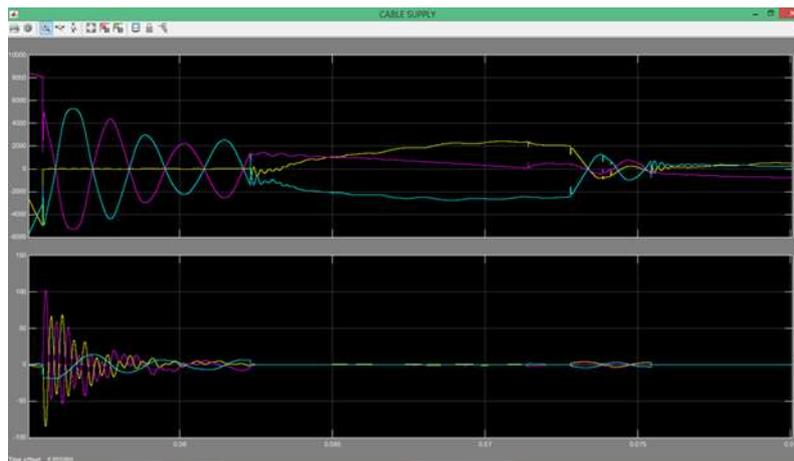
**Figure 3.2:** voltage and current supply to the transmission cables with load
