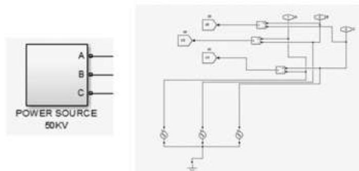
**Figure 2.2:** power source model from matlab simulink model
