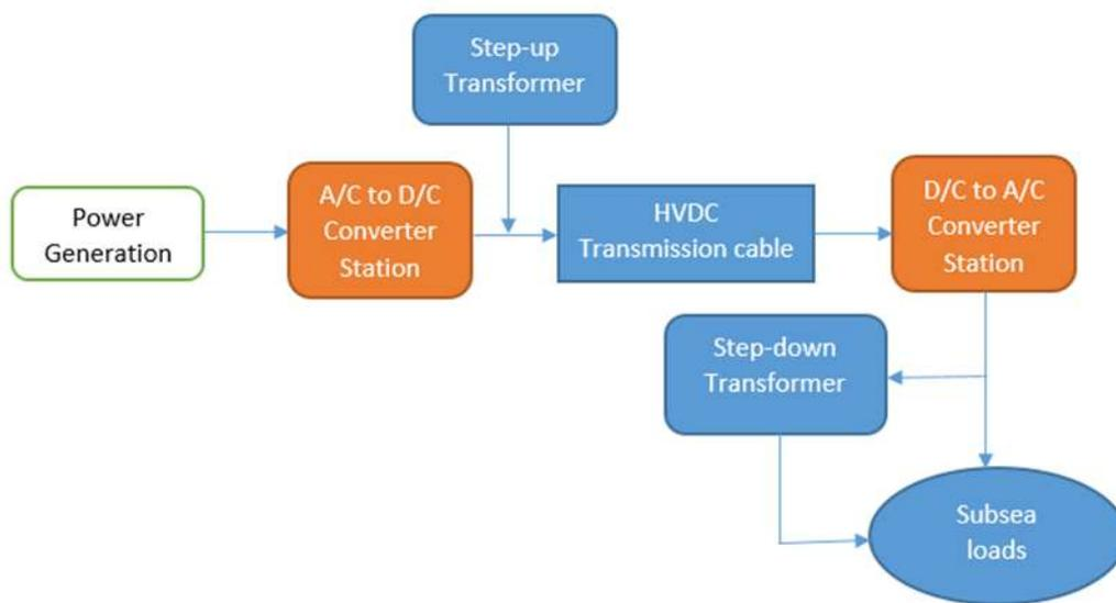
**Figure 2.1:** the modular subsea direct current system concept (source: [8]).
