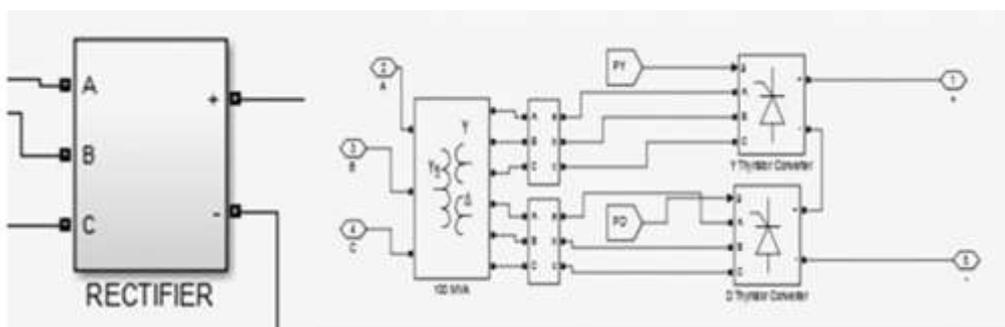
**Figure 2.5:** the rectifier block from matlab simulink model
