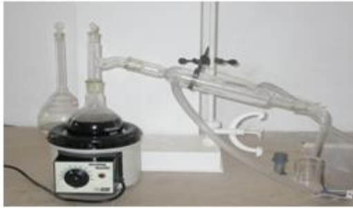
Fig.1 Experimental Setup for the Production of Esterified Oils Fig.2 Separator Funnel
