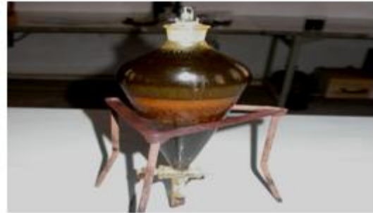
Fig.1 Experimental Setup for the Production of Esterified Oils Fig.2 Separator Funnel
