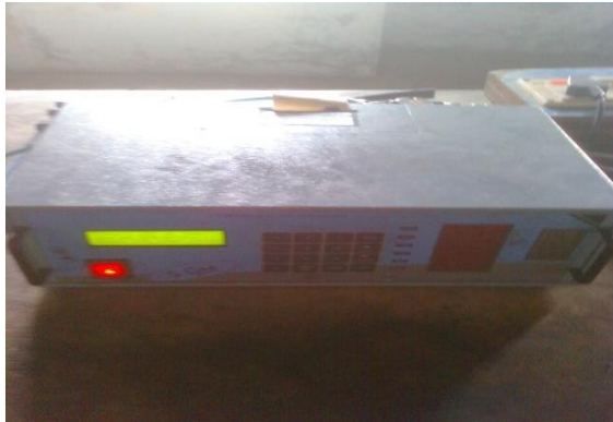
Fig.4 EXHAUST GAS ANALYZER
