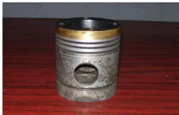
Fig.6 ALUMINUM PISTON WITH BRONZE CROWN
