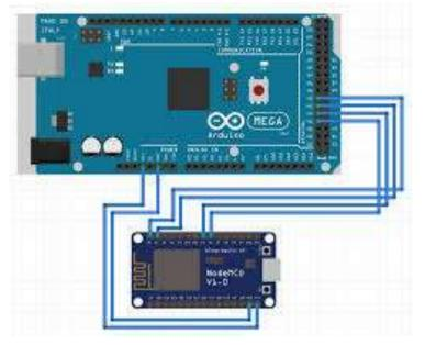
NodeMCU is great for connecting cloud and arduino is great at talking with different sensors. nodemcu has only one analog pin. Arduino will take analog readings and send the readings to nodemcu over serial connection. Nodemcu will send message for every reading it receives.
