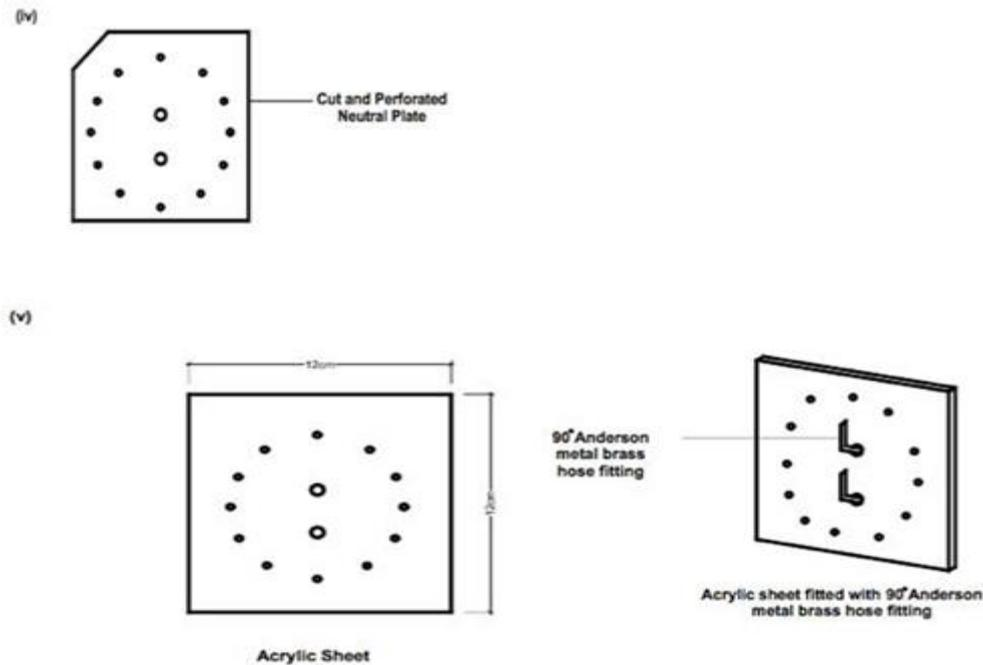
Figure 1. Cuts components of HHO generator
