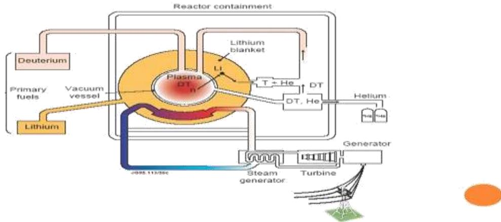
Fig 1. Working of ITER
