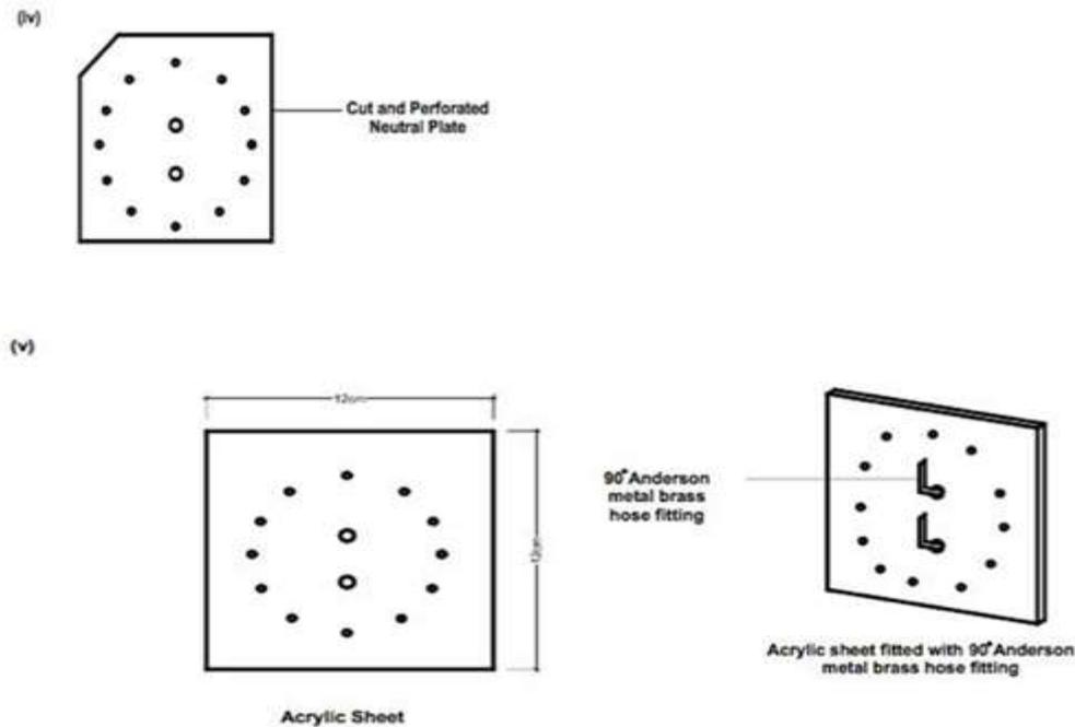
Figure 1. Cuts components of HHO generator
