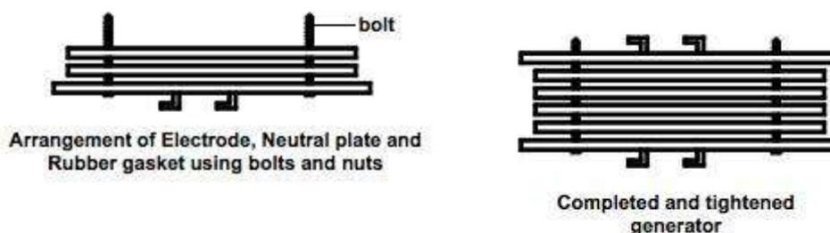
Figure 2. The step-wisearrangement of the oxyhydrogen generator electrode plates
