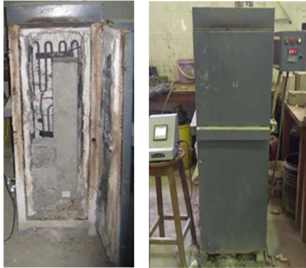
Fig. 4. Column inside the electric furnace ready for heating.
