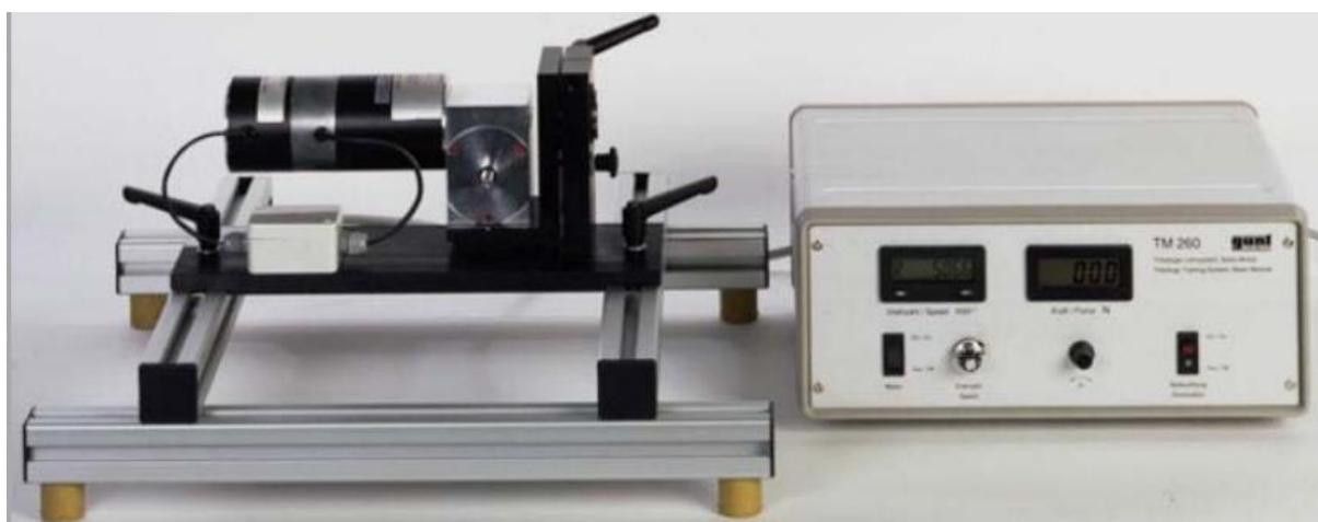
**Fig 3.1: TM 260.01 Rolling and Sliding Disc Tribometer [13].**
