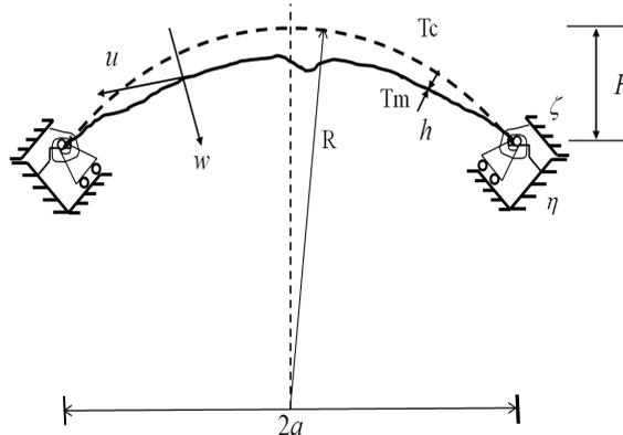
**Fig. 1** Geometrical model of FGM shallow spherical shells
