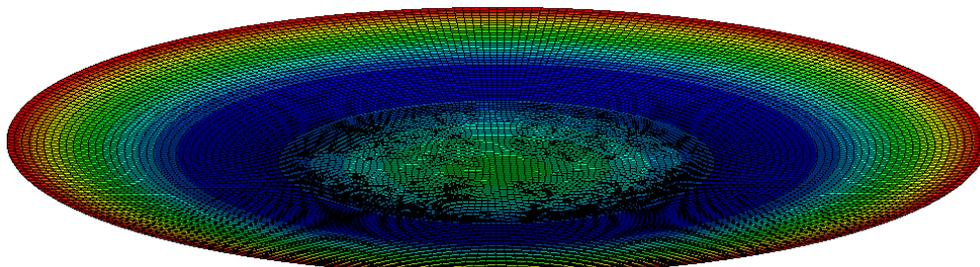
**Fig. 3** Snap-through buckling deformation of FGM shallow spherical shells
