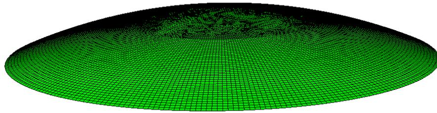
**Fig. 2** Finite element model of FGM shallow spherical shells
