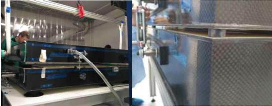
**Figure 4:** Left: Table II on top of Table I during drift panel construction. Right: The precision spacers between the two tables.
