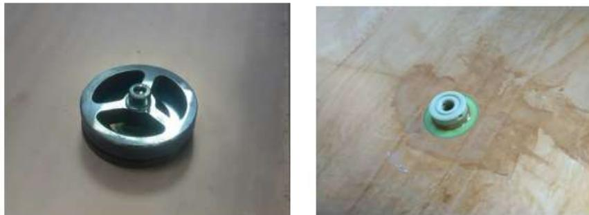
**Figure 5:** Left: The special tool developed for the interconnections spacers gluing. Right: The interconnection spacer after gluing.
