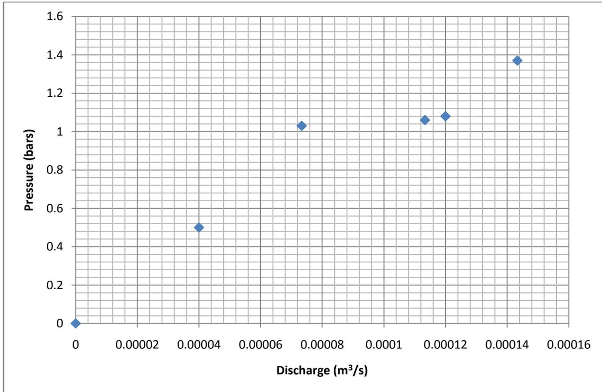
Figure 4.3: Shows the variation of Pressure with the Discharge of the Tablespoon Pelton wheel turbine
