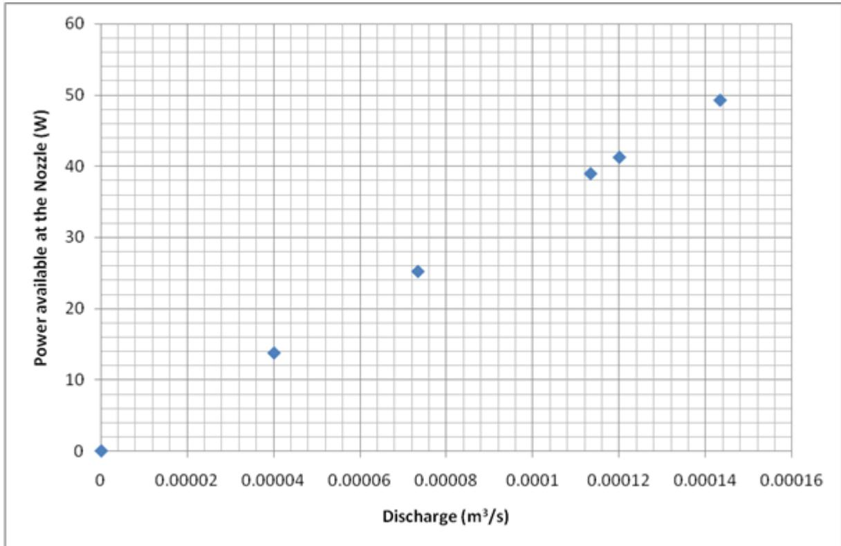
**Figure: 4.4:** Graph of Power available at the nozzle against Discharge of the turbine
