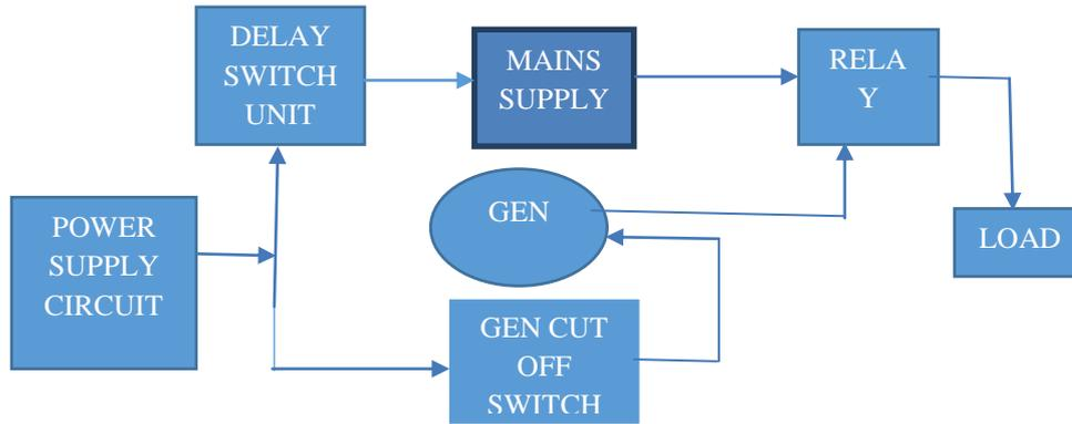
Figure 1 Conceptual Block Diagram of the proposed Automatic Change-over Switch
