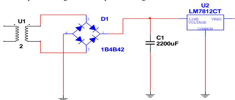
Figure 3 Power Supply Unit using Center-Tapped Transformer
