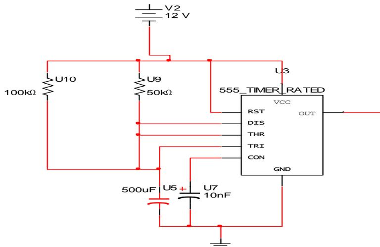
Figure. 5 The schematic diagram of the Astable 555 timer
